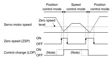
Note: When ZSP is not on, control cannot be changed if LOP is switched on-off. If ZSP switches on after that, control cannot not be changed.
